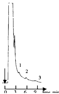
Fig. 2. Laboratory standard culture, 20 th day of laboratory cultivation. 1. Nerol 2. \beta -phenylethyl alcohol 3. Eugenol
